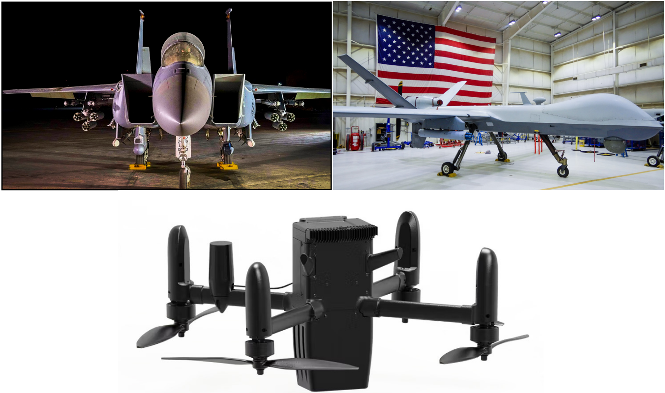
Figure 4: Two promising cost-effective C-sUAV effectors are AGR-20F Advanced Precision Kill Weapon System II laser-guided rockets, loaded on either F-15E Strike Eagles or MQ-9 Reapers, and Anvil drone interceptors.
