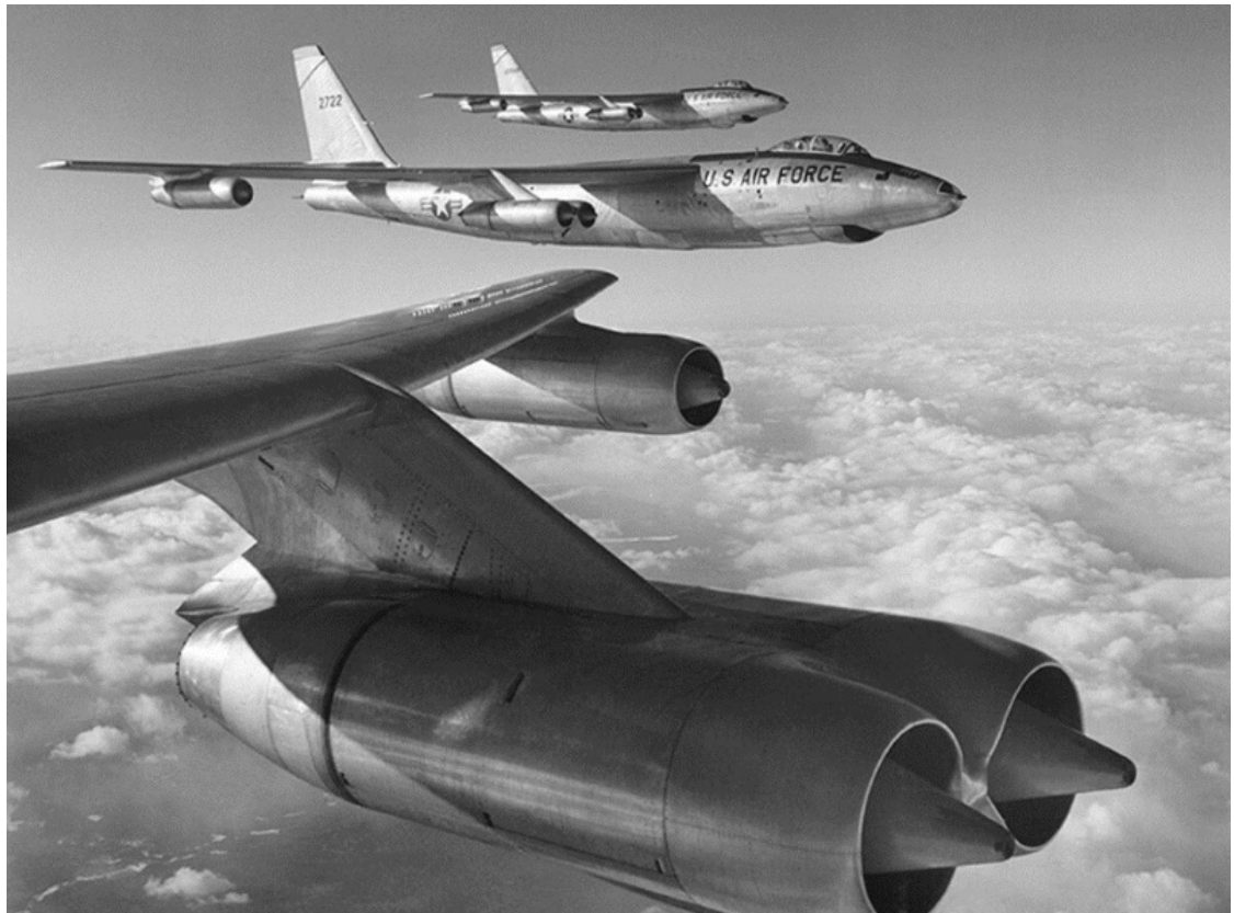
Figure 1. B-47s in formation. B-47s were designed with swept wings and turbojet engines to ensure they could match the inflight speeds of jet-powered fighter interceptors.
