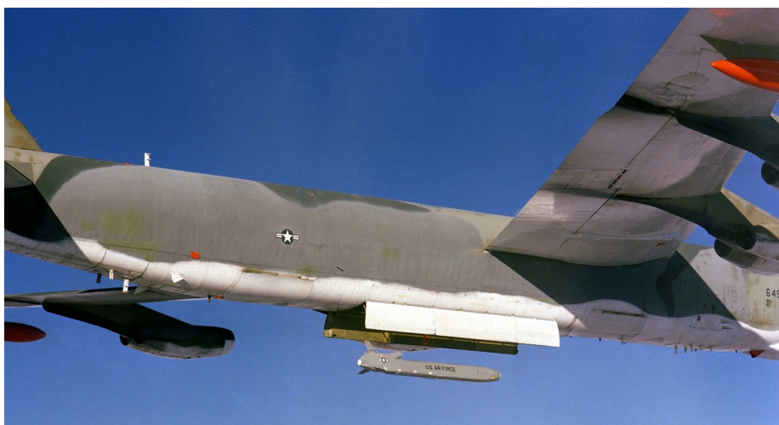
Figure 2. B-52 launching an AGM-86 ALCM. Designed for an operational life of ten years, ALCMs remain the Air Force's only nuclear-capable cruise missile over 40 years since joining the inventory. The stealthy Long-Range Standoff Missile will replace the ALCM.
