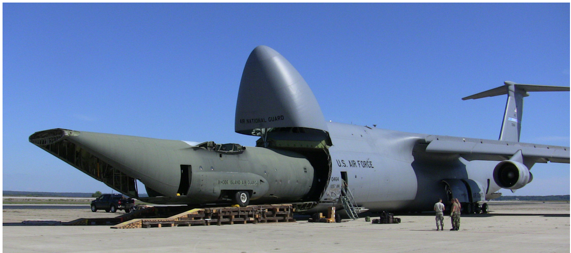
Figure 4: As the photo shows, a C-130 trainign fuselage can be loaded onto a C-5 for transport. Varying sizes of mobility aircraft afford different challenges and opportunities depending on mission requirements.
