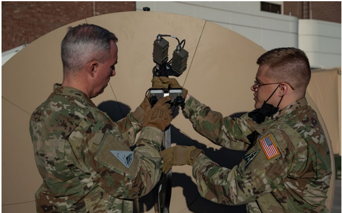
Figure 3: A USSF Guardian from Space Delta 3 – electromagnetic warfare, demonstrates a feed swap on a Giggasat FA-150 antenna at Peterson Space Force Base, CO. The antenna is used to aid in detecting and identifying electromagnetic interference, and Space Delta 3 is one of two provisional Integrated Mission Deltas stood-up to strengthen unity of command for readiness and promote unity of effort for capability development.
