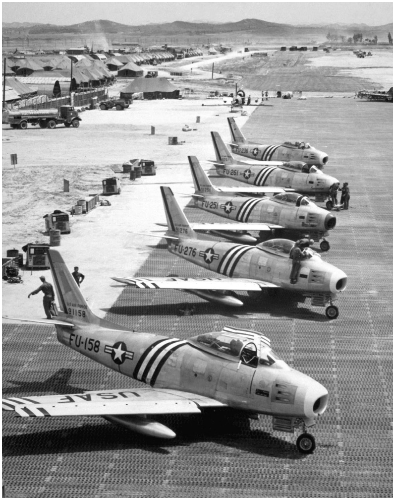
Figure 6: F-86s forward-based on a pierced steel plate ramp with little defense against attack or shelter to facilitate maintenance. Credit: U.S. Armed Forces Photo
