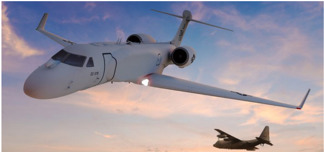
The new EC-37B Compass Call electronic warfare aircraft with an EC-130 in the background
