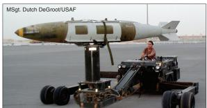
Above: A weapons loader prepares a GBU-31 Joint Direct Attack Munition for a B-1B sortie at a location in Southwest Asia. A Vietnam War-era Mk 84 bomb fitted with a GPS kit, despite advances in precision and accuracy, the essential components and bomb body of the GBU-31 have only marginally changed in the decades since the "Mark 80" series of general purpose munitions first debuted in combat.
