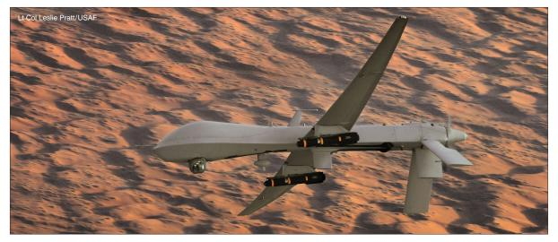
Above: An MQ-1 Predator, armed with AGM-114 Hellfire missiles, flies a combat sortie over Afghanistan. By merging sensors and munitions on one airframe, the US marked a new era in warfare beginning in late 2001. Targets could be observed and prosecuted rapidly—in many instances, measured by minutes—instead of determined far in advance.
