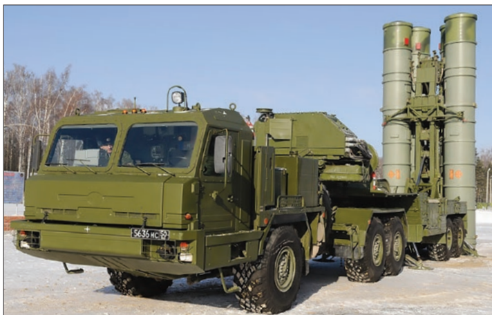
Left and below: The mobile multi-channel anti-aircraft missile system S-400 "Triumph" is designated in the West as the SA-21 SAM. Its main components include the 5P85TE2 TEL (at left) and the 92N6E Grave Stone Multimode Engagement Radar (pictured below). (Almaz)
