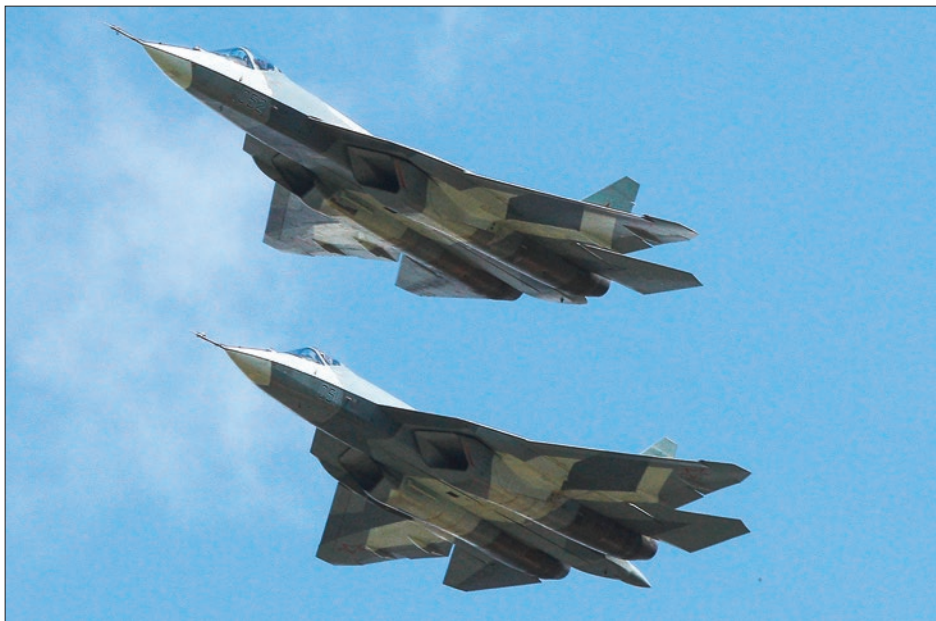
Left: A pair of Russia's Sukhoi T-50 PAK-FA prototypes during a display. The aircraft is claimed to have a radar signature of three to four square feet. (Sukhoi)
